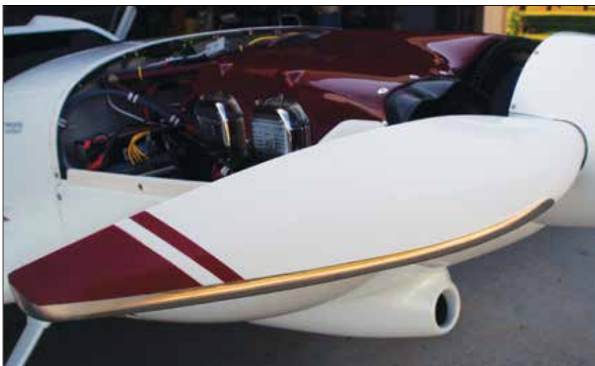
A two-blade composite WhirlWind ground-adjustable propeller provides the appropriate thrust.
