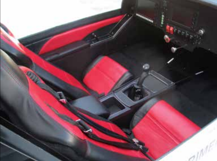
(Left) The demonstrator was nicely upholstered with red and black leather. The center stick frees up space, but dual sticks are also available. (Right) There's plenty of room for avionics on the panel. The demonstrator is equipped with MGL Avionics PFD and MFD displays.
