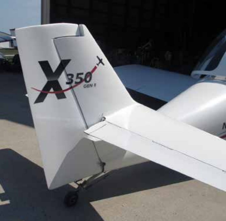
(Left) The one-piece vertical fin is molded into the upper section of the fuselage. The cruciform horizontal tail is mounted well above the wake from extended wing flaps. (Right) The elevator trim tabs on N181WA were fixed, but adjustable electric trim is being considered for future kits.
