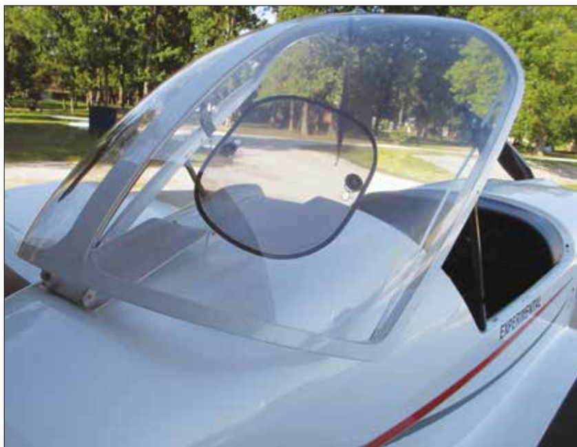
The articulated lift-up canopy swings fully aft over the turtle deck to give unrestricted access from either wing walk.
