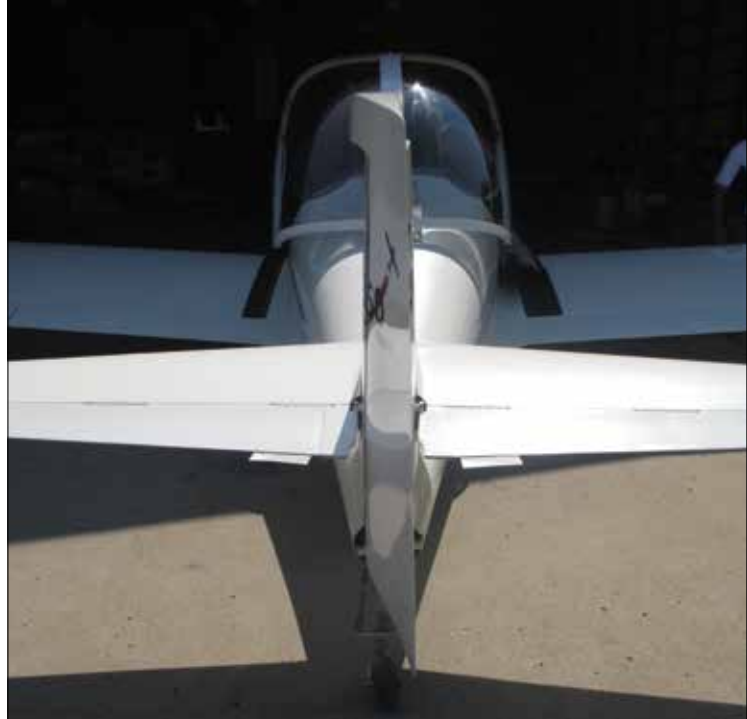
(Left) The one-piece vertical fin is molded into the upper section of the fuselage. The cruciform horizontal tail is mounted well above the wake from extended wing flaps. (Right) The elevator trim tabs on N181WA were fixed, but adjustable electric trim is being considered for future kits.
