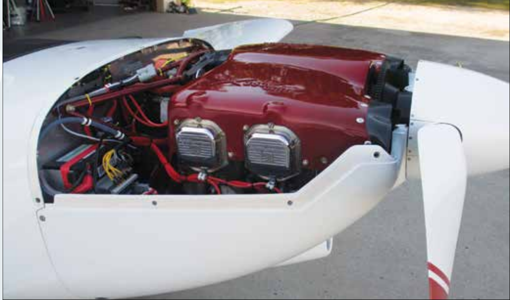
The Lycoming O-320 is fitted with Superior Millennium cylinders. A sleek plenum is used for cooling instead of a baffle system.
