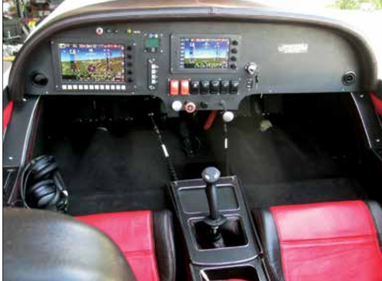
(Left) The demonstrator was nicely upholstered with red and black leather. The center stick frees up space, but dual sticks are also available. (Right) There's plenty of room for avionics on the panel. The demonstrator is equipped with MGL Avionics PFD and MFD displays.
